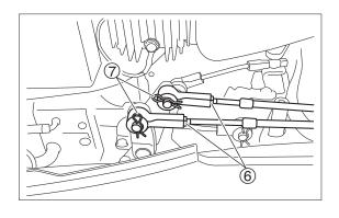
· Lock joint with nut ⑥ and secure with washer and R pin ⑦.
